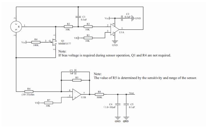
The diagram above is a recommended circuitry for three-electrode EC sensors. It consists of three parts: Potentiostatic Circuit, I/V (current/voltage) Converting Module and Short-Connected Configuration.
